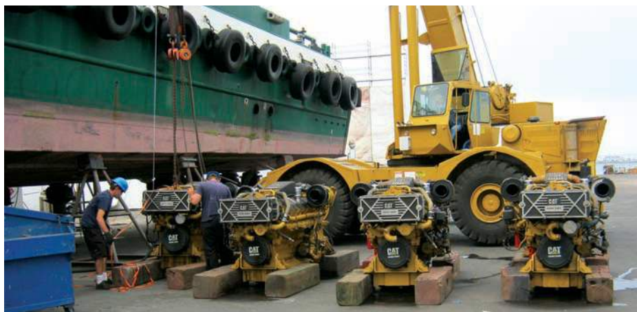
Marine Group workers remove the rigging from the last of four old engines to come off the Piper Inness .
