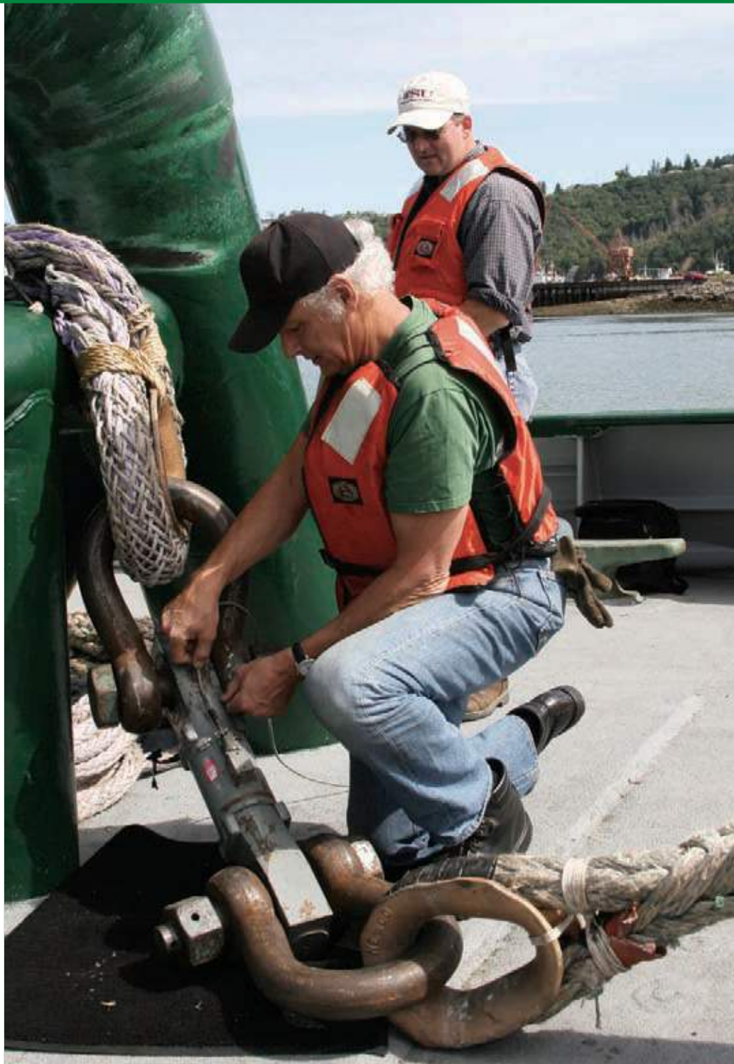
Altus rigs a load cell during a recent bollard-pull test for a Foss tug on Commencement Bay in Tacoma.
