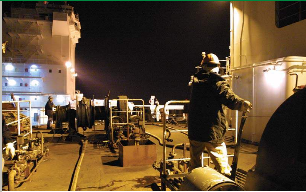
A worker on the Chevron tanker Cygnus Voyager , foreground, throws a lever activating one of the big winches that draw his ship together with the ultra-large crude carrier TI Africa .
