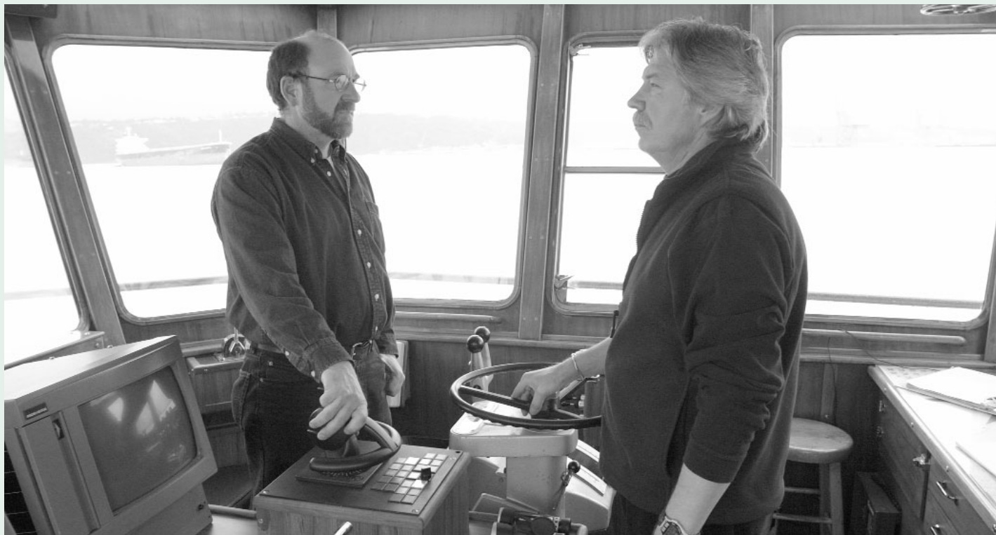
Captain Mike Blake , left, works the control for the new ASD drive on the Wedell Foss , while Captain Doug Hajek operates the control for the VSP units.
