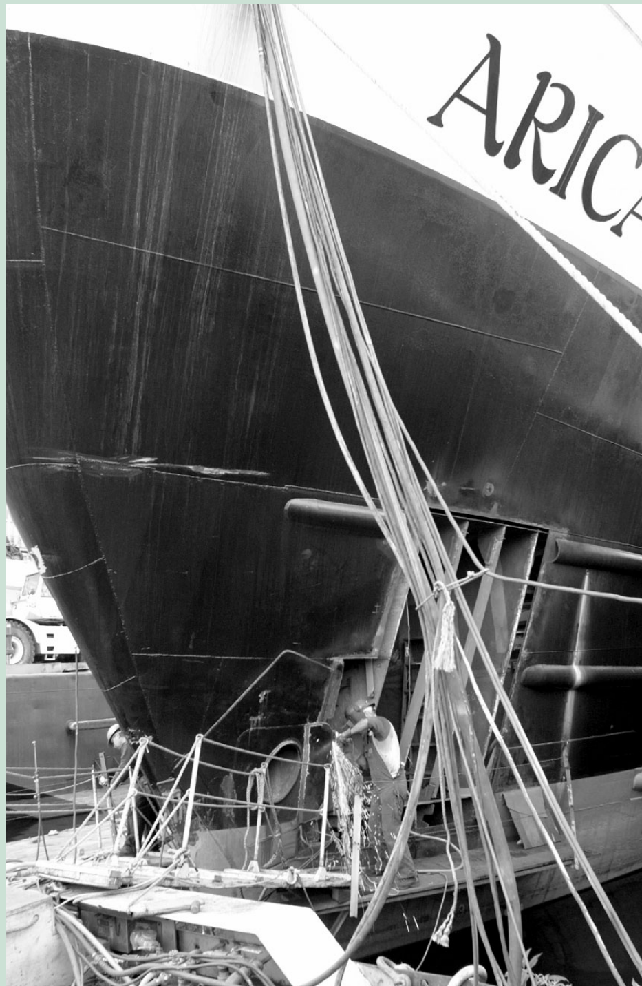
Replacing steel in the bow was among jobs performed this fall on the trawler Arica at Foss Shipyard.
