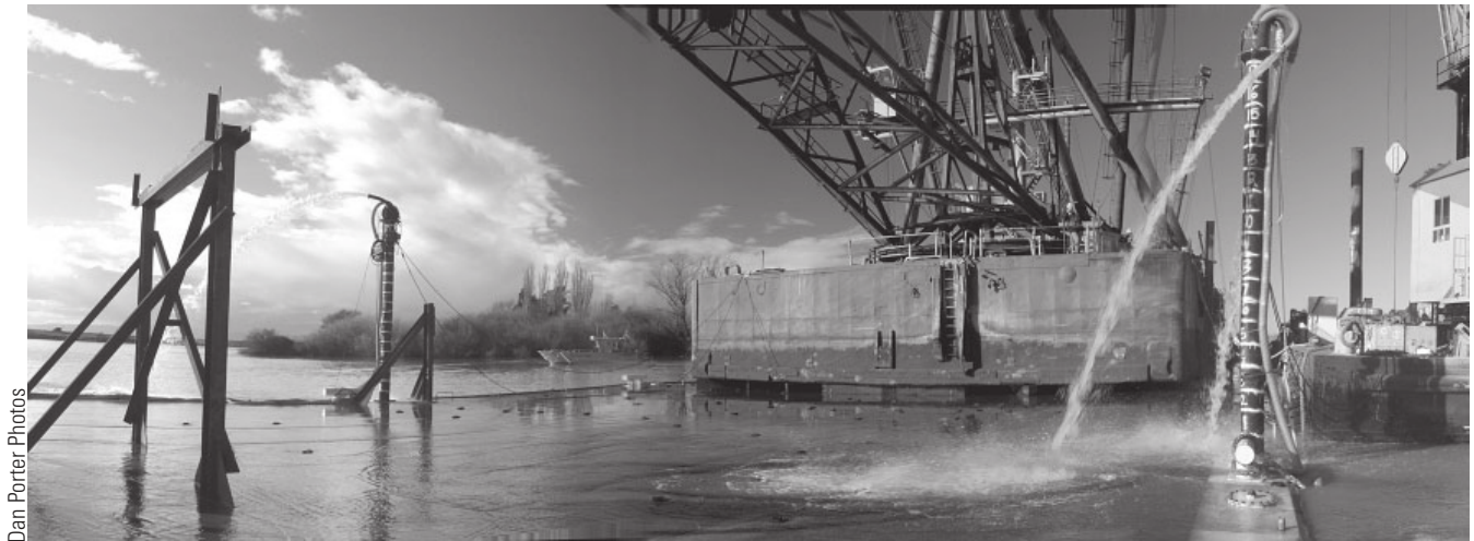
The deck of the submersible barge MZB287, with the Monarch on board, breaks the water as the pumps run full tilt.
