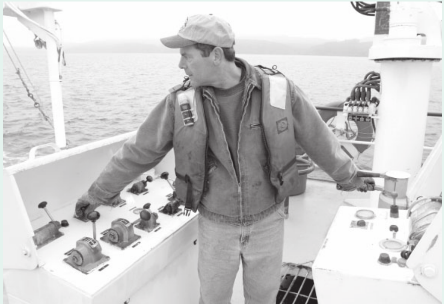
Mate Scott McKinley is at the controls on the boat deck of the Barbara Foss , trying to snag an “anchor chain” with the retrieval hook.
