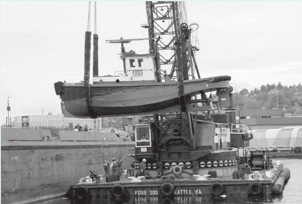
The Foss 300 derrick lifted the tug Sam Foss onto a barge in Seattle recently for transport to San Francisco Bay, where the 40-foot boat will help out in a variety of work areas.
