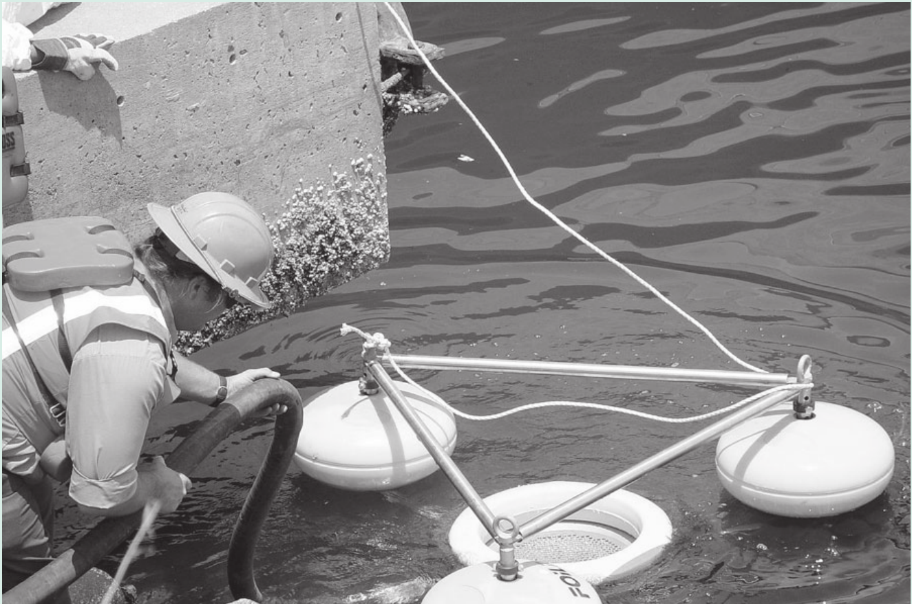
Jeff Edwards of Foss Environmental Services with a vacuum hose connected to a "Foilex Mini" suction skimmer.
