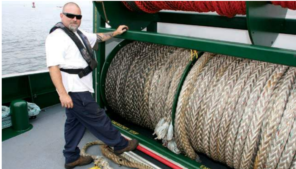
Allen Ryle demonstrates the emergency kick bar which can be used to shut down the Lucy's line reels if something or someone were to get caught in them.
