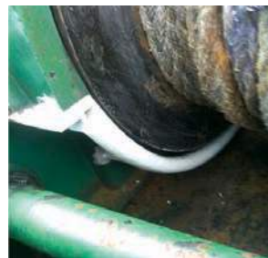
The white guard was added to prevent the towline from flipping off the winch drum.
