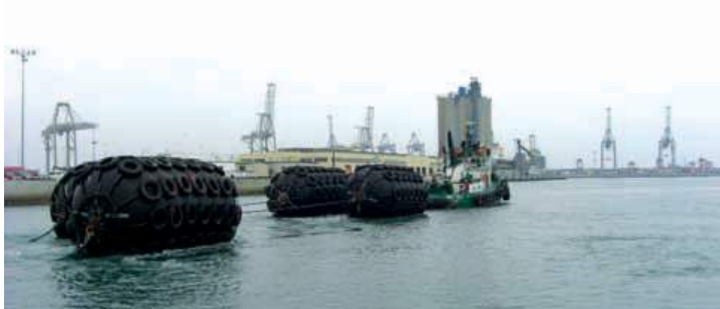
The Edith Foss has four big Yokohama fenders in tow as it heads for the Pacific Area Lightering (PAL) zone. The fenders are used to separate tankers during lightering operations.
