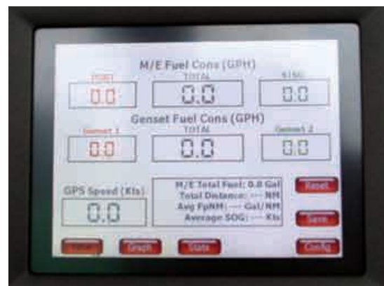
Engineer John Judd points to the flow detection devices on the fuel lines to one of the main engines. In the photo below, a display in the pilothouse of the Garth Foss keeps deck officers apprised of fuel consumption.
