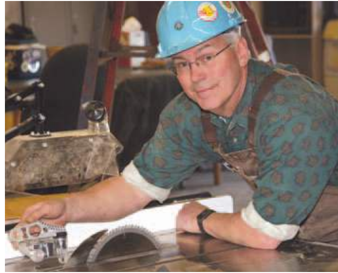
Assistant Shipwright Foreman Paul Paroline displays the braking mechanism that clamps against the underside of the saw blade when the blade comes into contact with skin.
