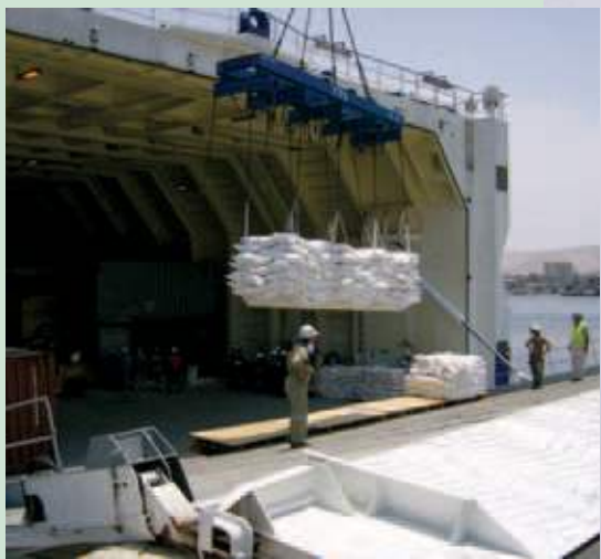
A top-pick machine, normally used to handle containers moves the food cargo to the pier.
