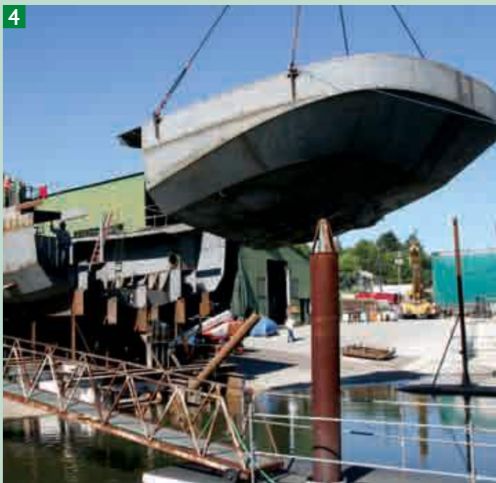
4 The stern section is moved into position on the ways, where it will be welded to the already-placed bow- and mid- sections.
