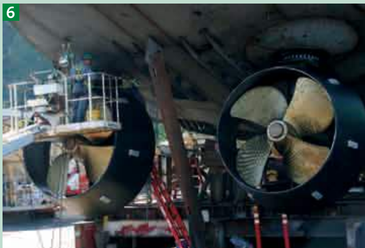
6 A shipyard worker, on the lift, puts the finishing touches on one of the drive units, installed on Sept. 8.
