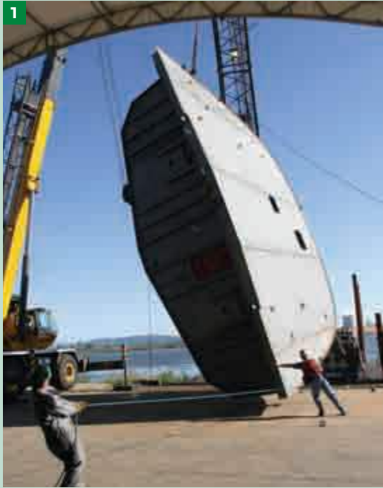
1 The 84,000-pound stern section of the tug, built upside down, is flipped in preparation for transport to the ship ways and union with the rest of the hull.
