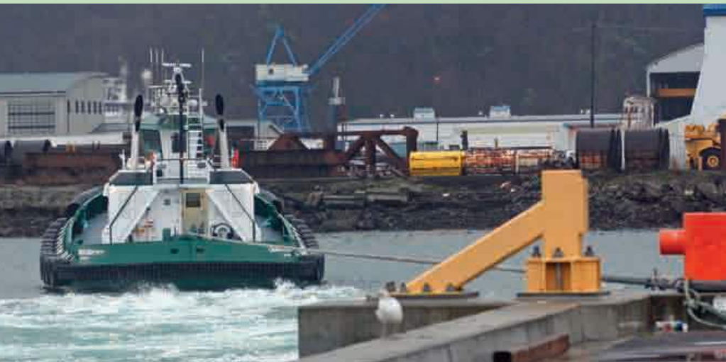
During a bollard-pull test on Jan. 6 in Tacoma, the Carolyn Dorothy's pulling power proved to be in the same range as its diesel-powered sisters.
