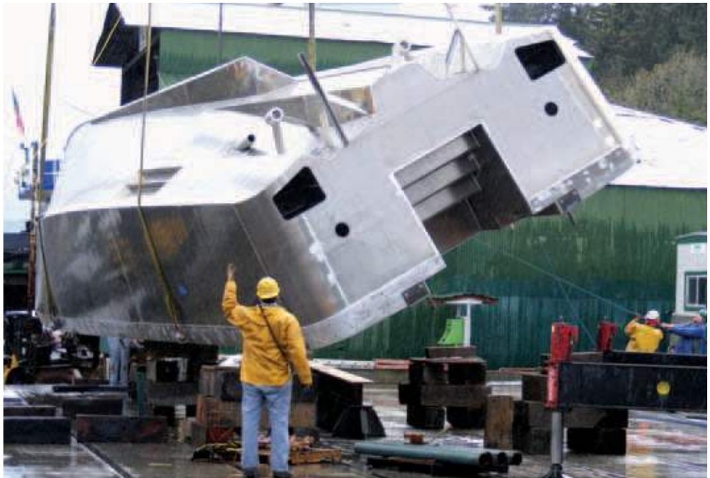
Cranes flipped the hull of the Ava Foss to an upright position on April 6 at Foss Rainier Shipyard.
