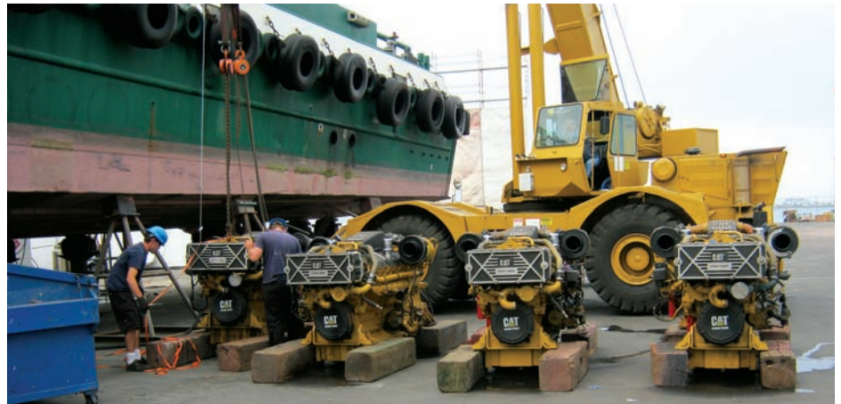
Marine Group workers remove the rigging from the last of four old engines to come off the Piper Inness .
