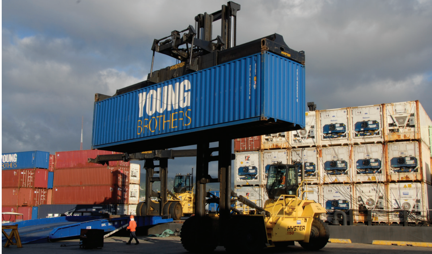
Young Brothers new top-lift machines can stack five-containers-high on the new barges, effectively increasing their capacity by 25 percent.
