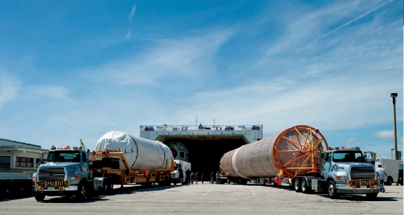
Trucks towed a Delta IV second stage, left, and an Atlas V booster from the cargo bay of the Delta Mariner at Cape Canaveral. Still on the ship is a Delta IV booster.
