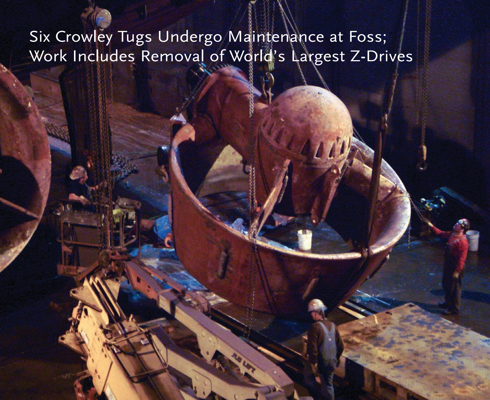
Foss Shipyard workers lower a 35-ton Z-Drive from the Crowley tug Attentive .
