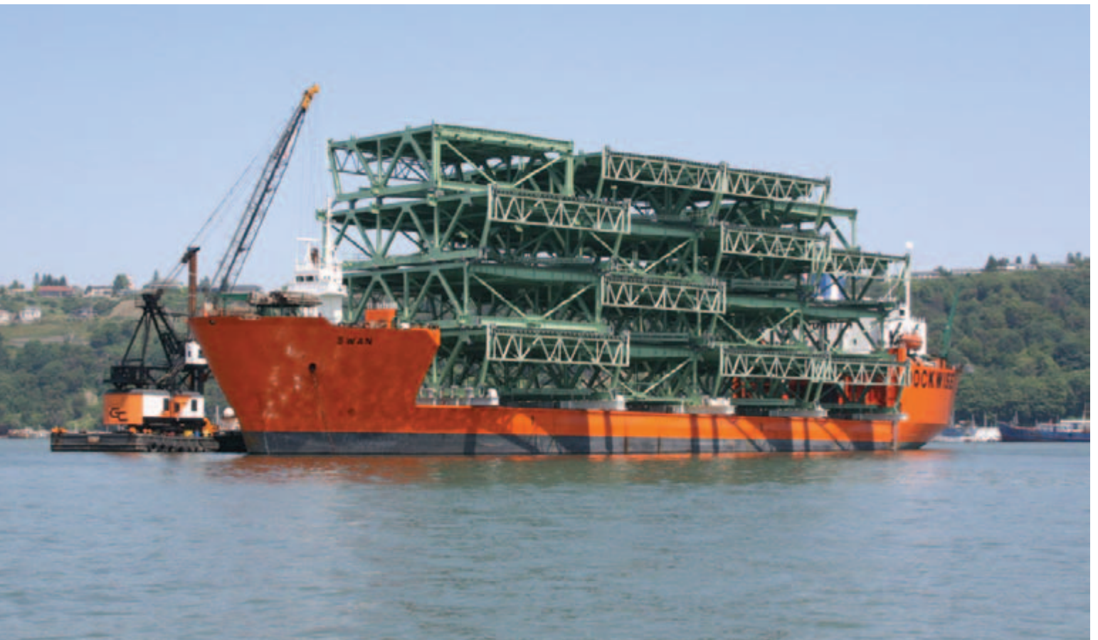
The heavy-lift ship Swan arrives in Tacoma’s Commencement Bay on June 8, carrying the first of three loads of roadway sections for the new Tacoma Narrows suspension bridge. Most of the sections are 120 feet long and weigh 450 tons, but the heaviest weigh about 600 tons.
