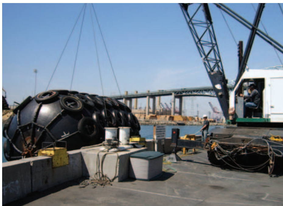
A big "Yokohama Fender" used to keep tankers apart during lightering is lifted onto the pier by Foss in Long Beach. Foss personnel maintain the fenders and other lightering equipment for Chevron Shipping.
