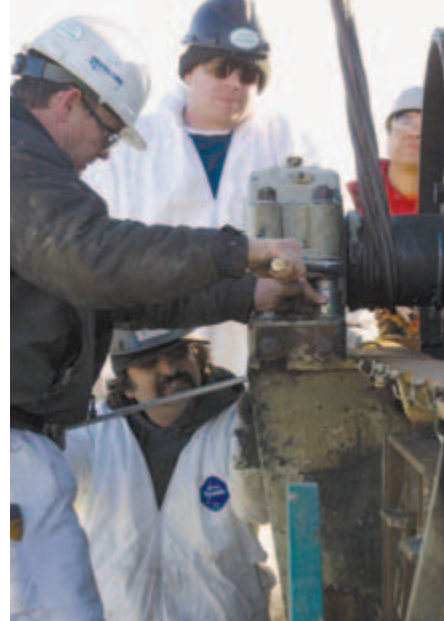
Ship Repair Superintendent Greg Schaut , left, supervises at Foss Shipyard as workers install the new "pocket belt." With him are barge crewmembers Brett Walker , turning the wrench, and Bogdan Fetsek , center, and Rigger Ramone Johnny , right.
