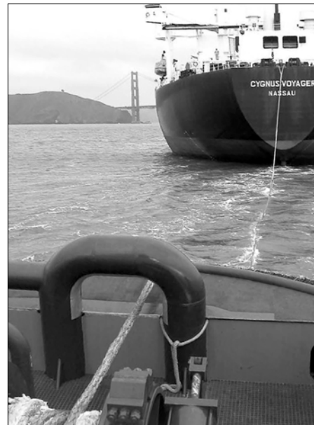
The system records line tension by measuring the load on the winch brake and transmitting the data to a computer in the pilothouse.
