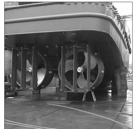
The Hoku Kea , shown in drydock at Foss Shipyard in the winter of 2005 after installation of new props, nozzles and triple-vane rudders.
