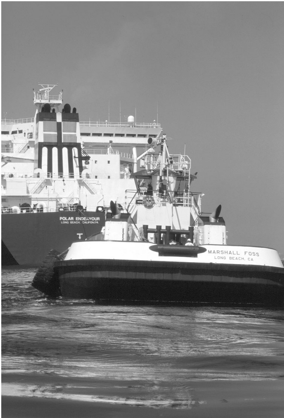
The Marshall Foss , shown during a tanker escort, is equipped with a tow winch and packs enough horsepower to double as an ocean tow boat.
