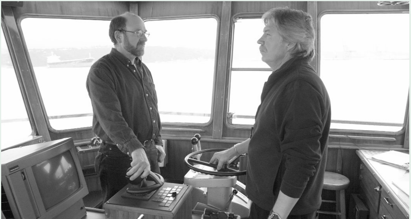
Captain Mike Blake , left, works the control for the new ASD drive on the Wedell Foss , while Captain Doug Hajek operates the control for the VSP units.
