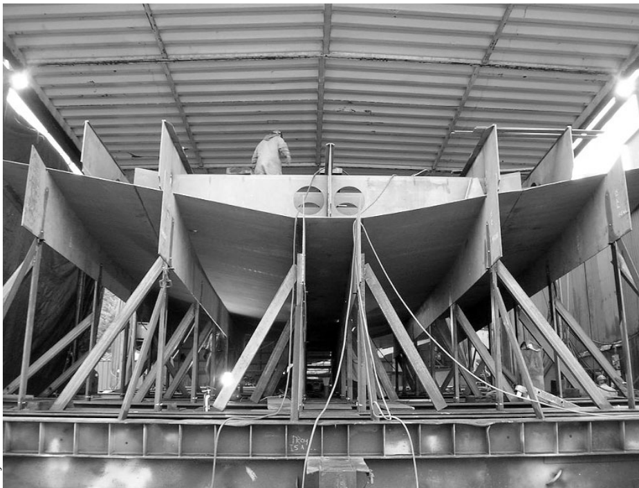
The mid-body section of a new Dolphin-Class tug is under construction on the large ways at the Foss Rainier Shipyard.
