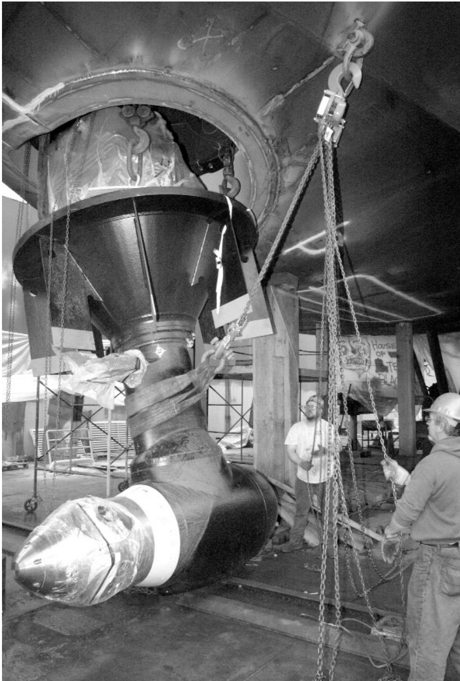
Rigger Terry Dawley, left, and Rigger Foreman Jim Mosman maneuver a new ASD drive into position under the stern of the Wedell Foss on December 2 at Foss Shipyard. The drive weighs 39,000 pounds.
