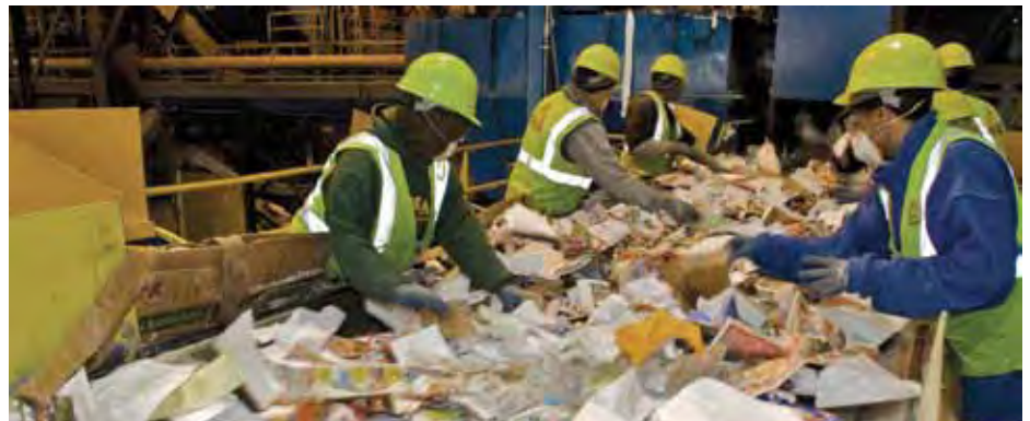
Allied Waste's South Seattle plant is crisscrossed with conveyor belts carrying mixed up recyclables. Workers line the conveyors and separate the materials.
