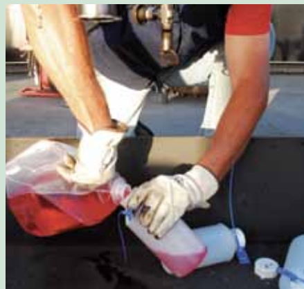
Harold Presswood takes a clean diesel sample to send to a test center for inspection.
