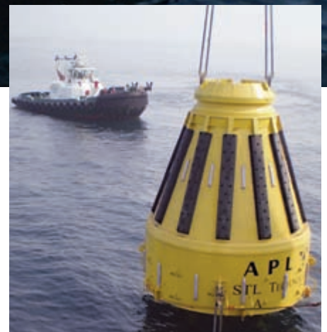
The Leo stands by as a subsurface buoy is lowered into the water.
