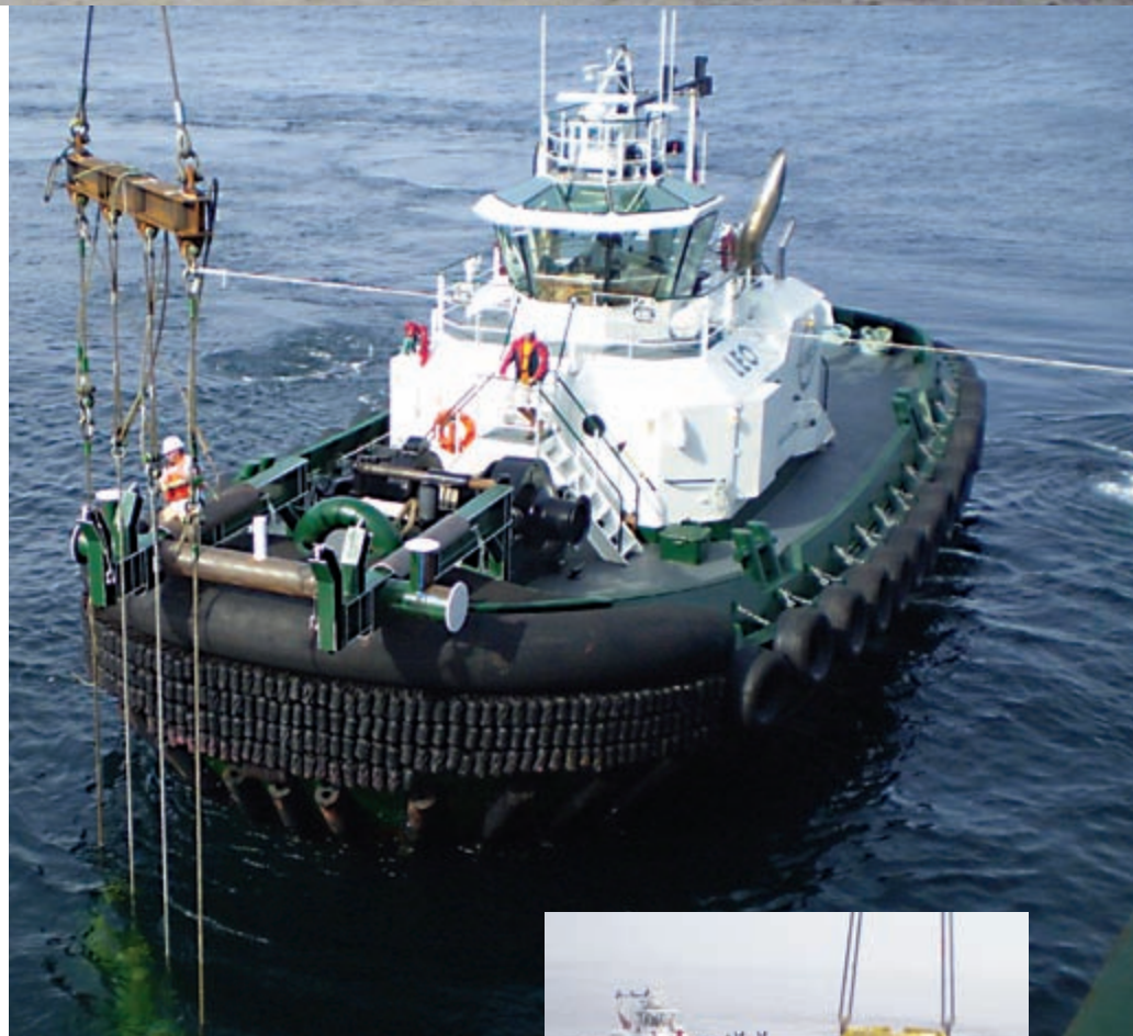
A beam attached to four anchor wires is lowered toward a framework built on the bow of the Dolphin-Class tug Leo .
