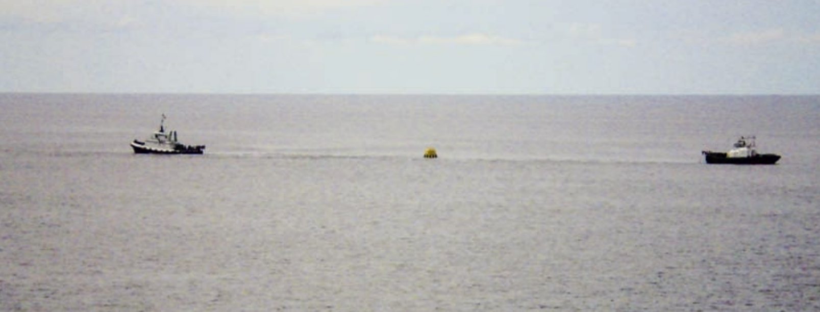
The tractor tugs Orion , left, and Leo maintain tension on the anchor lines attached to the subsurface buoy.
